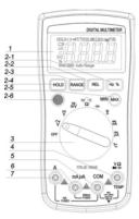
2-3 RANGE key: This key is used for selection of automatic or manual range. The instrument is in the state of automatic range initially, and shows the sign "AUTO". After this functional switch is pressed, it will turn into manual range. The level will be increased by one every time when the key is pressed, and it will recycle from low to high in turn. After the key is pressed for more than 2s continuously, the product will return to the state of automatic range;
