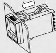
To push the clamp of special structure design without using screw to the end can be smoothly fixed on the panel.
